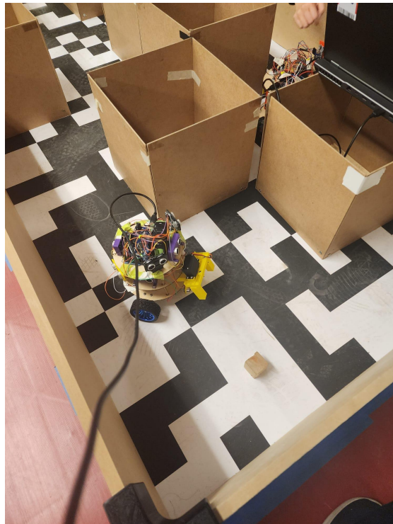
Figure 10: Detecting the block to pick it up. Notice the bias it has
